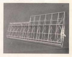
ated to guarantee maximum strength. The ribs and leading edge are constructed of corrosion-resistant Nicraluminum, a material that possesses a much higher strength factor than less modern constructions of plywood, as used in some ships. Finest obtainable spruce spars are treated with three coats of varnish, and fibre bushings are used at points of high loading. Many vitally important and expensive construction methods are employed for your complete security.
