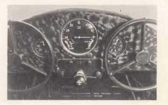
Switch, Throttle, Primer, Push-pull Gas Shut Off and Parking Brake Control. Chrome plated wheel shafts are also standard equipment.
